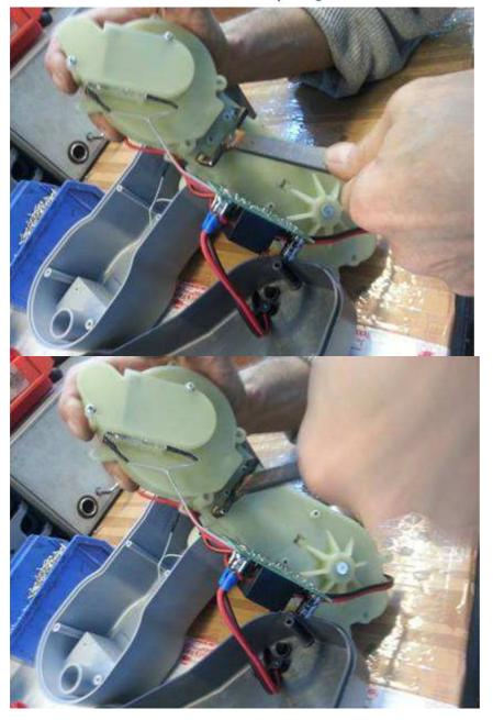
Remove and replace the piston/gear block:
