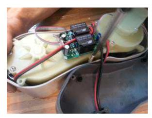
Then unscrew the 4 screws on the circuit board, as following:
