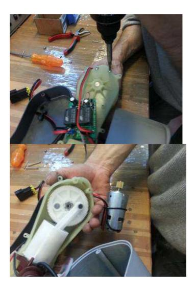
Separate the piston/gear block from its plastic seat by pushing simultaneously the tabs below:
