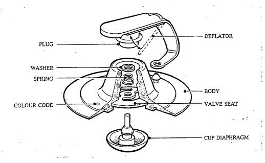
A4 valves are moulded in rubber or Neoprene, each indicated by a colour code on the valve body (red for rubber and yellow for Neoprene). Rubber valves are suitable for conditions between -40°C and +80°C, Neoprene for -20°C to +80°C.
